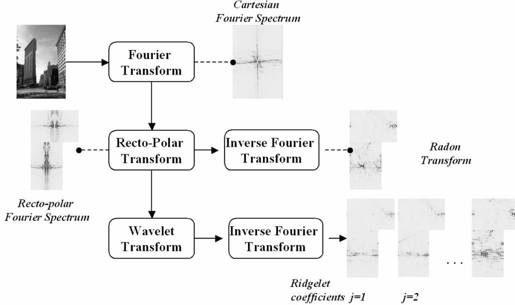
Fig. 3. Block diagram of the ridgelet forward transform
