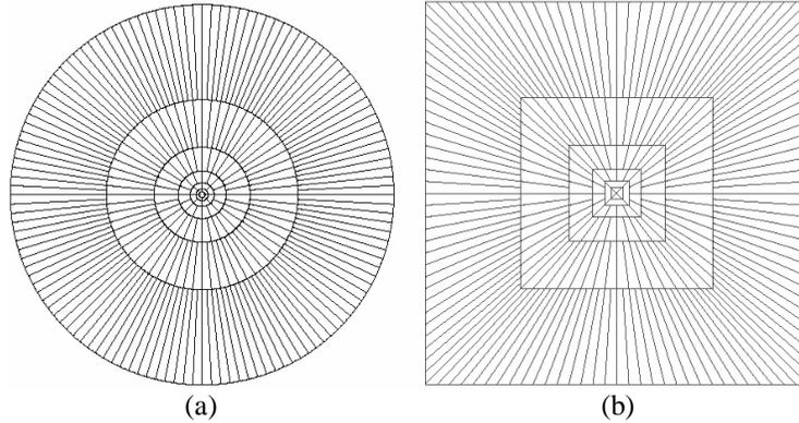
Fig. 1. a) Ridgelet tiling of the frequency domain and b) Digital ridgelet tiling (from [3])
