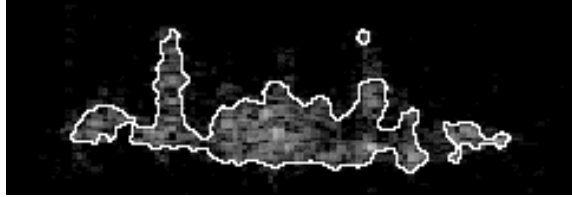
Figure 9: Final snake configuration for an experiment of target segmentation in ISAR images
