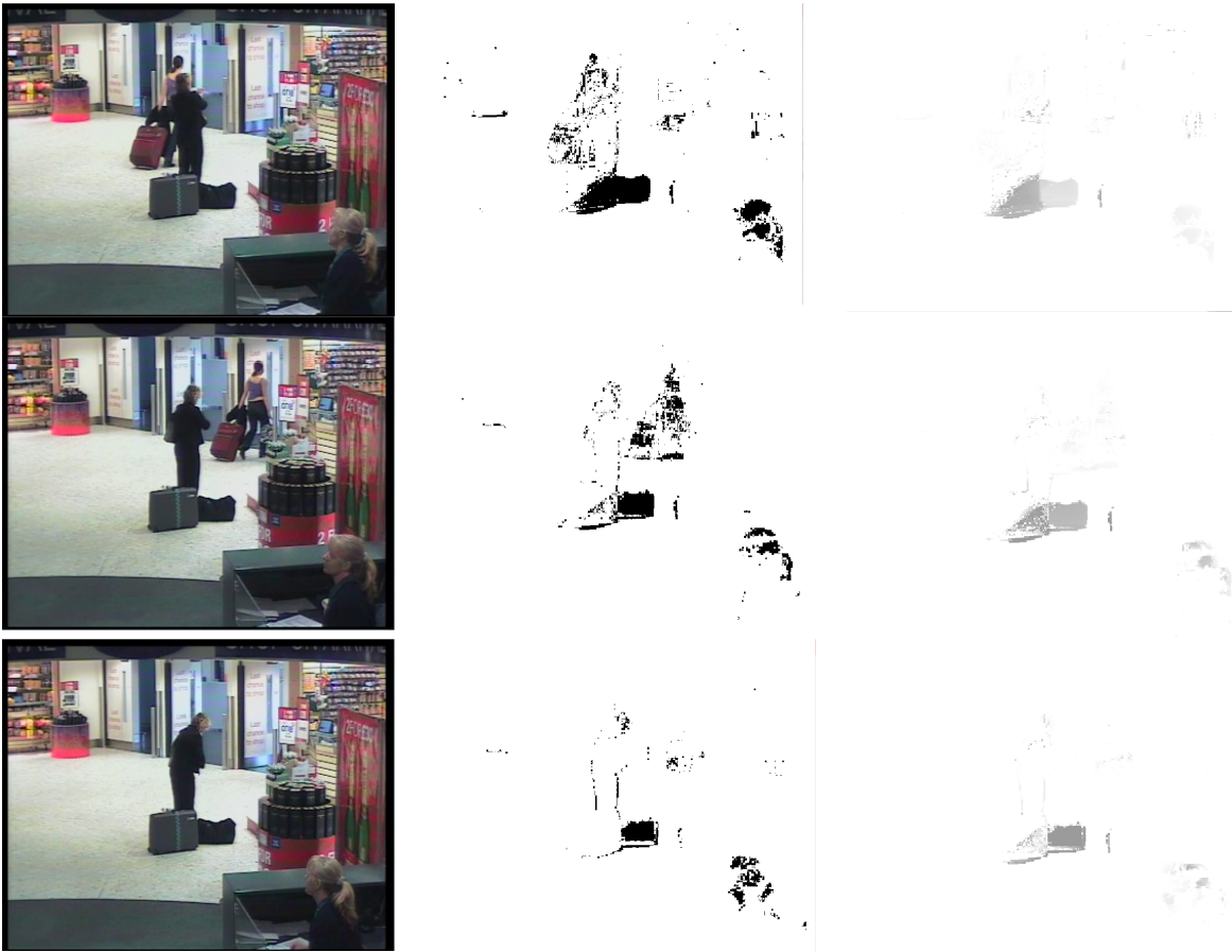
Figure 4: Some frames for an ObjectPut event (left column); foreground difference image (center) and alert images (left)
