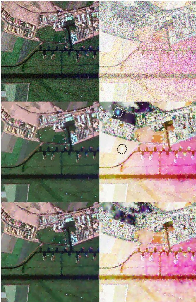
Figure 2. Filtering results on the E-SAR: The left column shows the master image ( $C^{11}$ ) and the left column is a color composite of the InSAR coherency maps ( $R = K_{hv}^{12}, G = K_{vv}^{12}, B = K_{hh}^{12}$ ). From top to bottom: Original Image; Yu Filter (1,500 iterations) and proposed method with the 6 power bands (465 iterations,  $a_+ = 2, a_- = 1.5, \Delta t = 0.05, M=2$ ).
