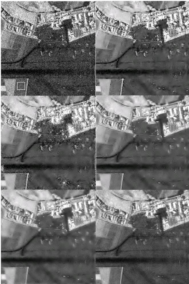
Figure 5. Results on the E-SAR image (HH), from left to right and top to bottom (in dB): original, SWT-MMSE, SCT-MMSE, SWT-Soft, SCT-Soft and Curv-Soft
