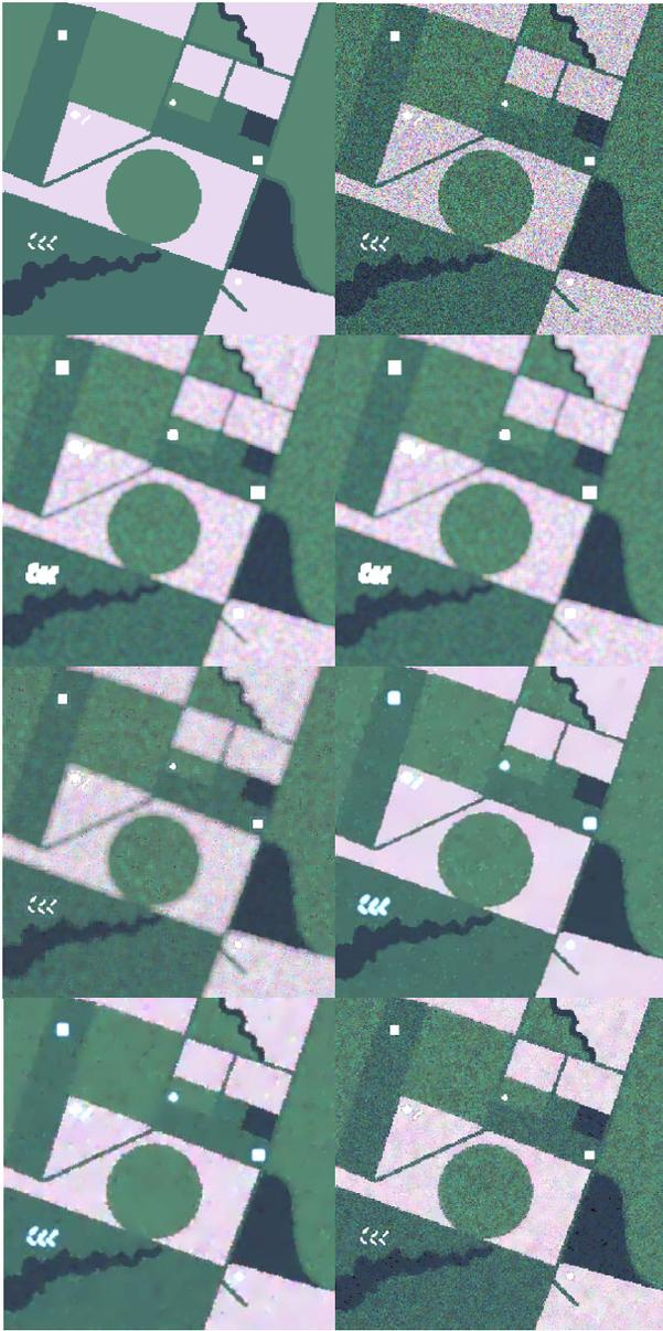
Figure 2. Span display color, red =  $\sqrt{2} |Shv|^2$ , green =  $|Svv|^2$ , blue =  $|Shh|^2$ , and from left to right and top to bottom : ground truth, original image, box filter, enhanced Lee, Subspace, Yu, Trace, SMB.
