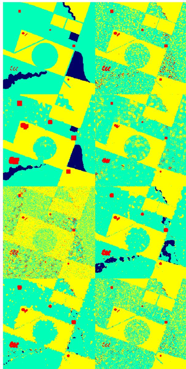
Figure 1. Classification of the dominant scattering mechanism based on Freeman Durden Decomposition, blue = undetermined, green = surface, yellow = volume, red = double bounce, and from left to right and top to bottom : ground truth, original image, box filter, enhanced Lee, Subspace, Yu, Trace, SMB.
