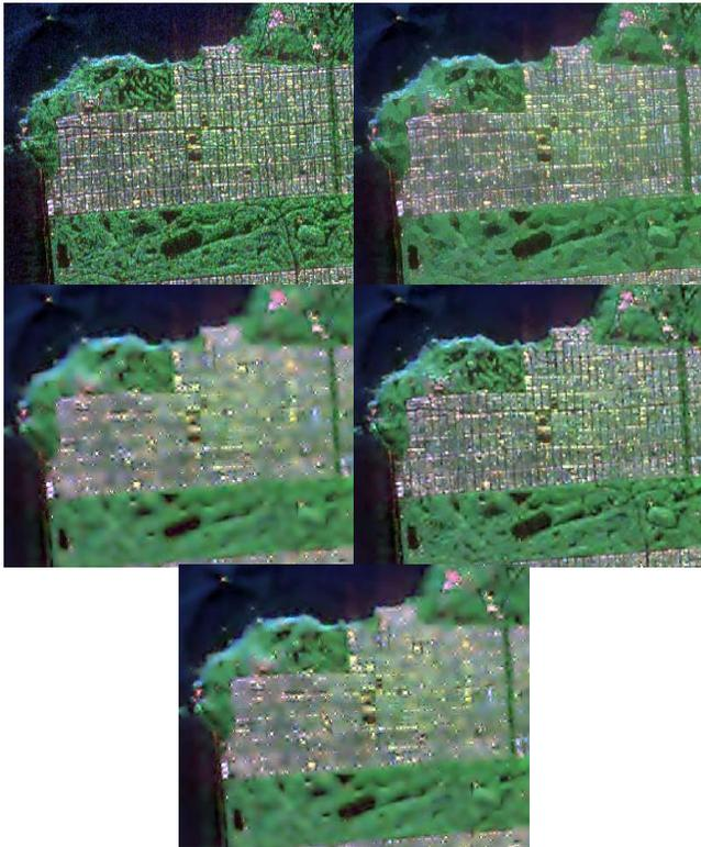
Figure 4. Display is obtained by a Pauli decomposition, and from left to right and top to bottom : original image, enhanced Lee (9x9), PCA on all bands with 3 levels, SSC on all bands with 4 levels, power bands with 3 levels.
