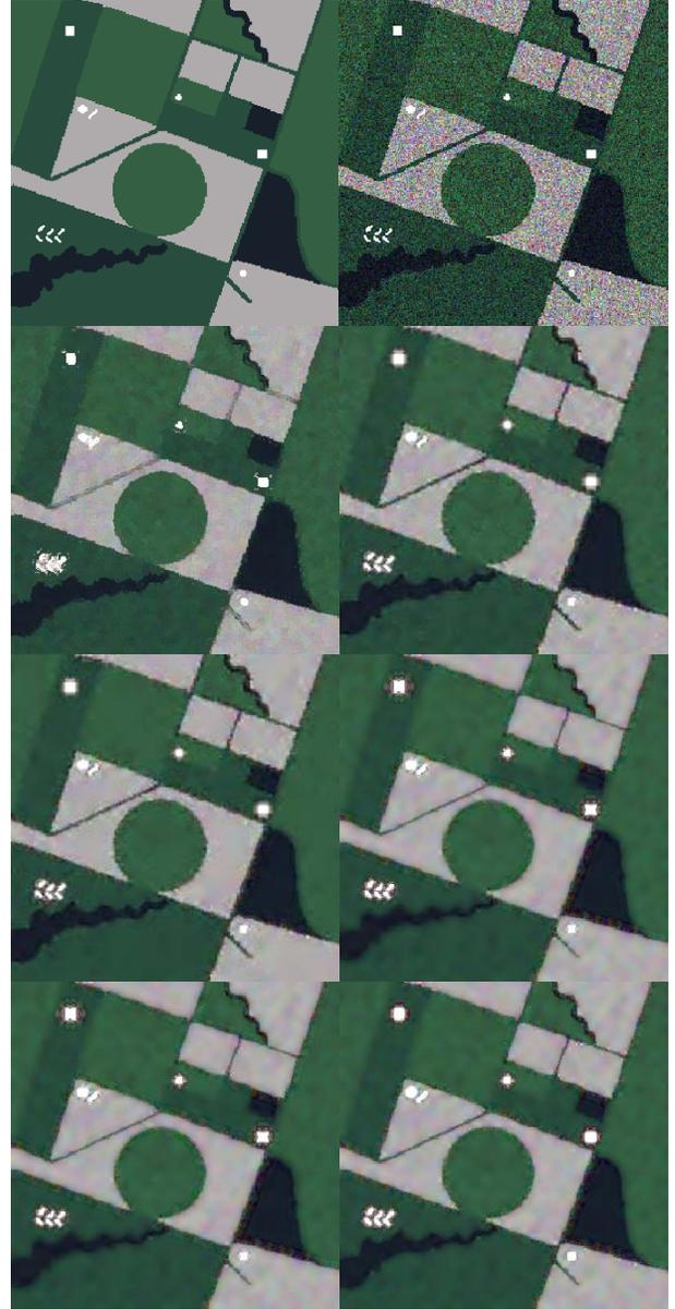
Figure 3. Display color, red =  $\sqrt{2} |Shv|^2$ , green =  $|Svv|^2$ , blue =  $|Shh|^2$ , and from left to right and top to bottom : ground truth, original image, enhanced Lee (9x9), SSC on all bands with 4 levels, SSC on all bands with 3 levels, PCA on all bands with 3 levels, PCA on all bands with 4 levels, power bands with 4 levels.
