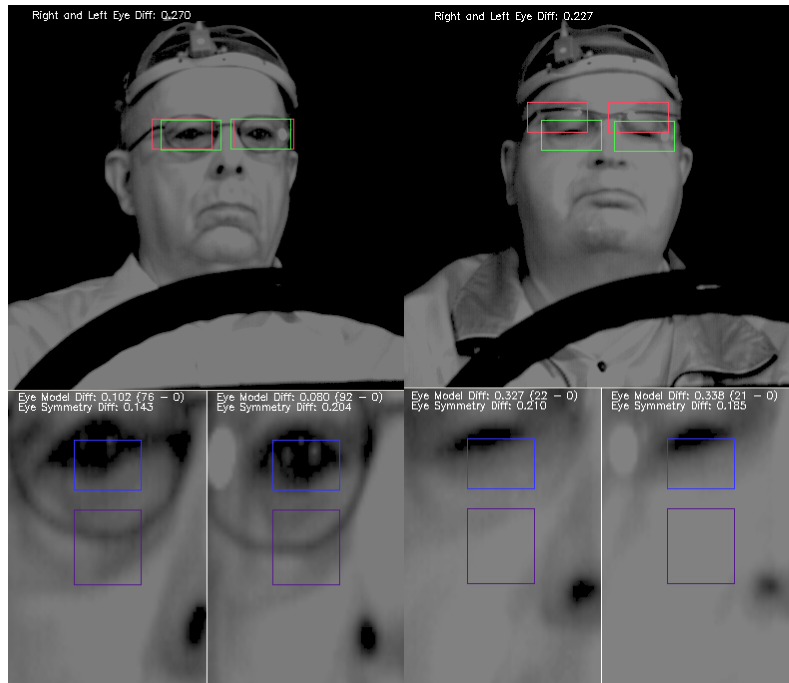
Figure 1. In the upper images, red boxes show the approximate eyes position based on image profiles and the green ones are the best positions found. The lower images show left and right eye regions with the desired eye location in light blue. The ROI will be well aligned with the pupil when the number of dark pixels in the light blue box/violet box are maximal/minimal. Note that the images shown here, as well as in the remainder of the paper, have been enhanced (histogram-equalized) for clarity.
