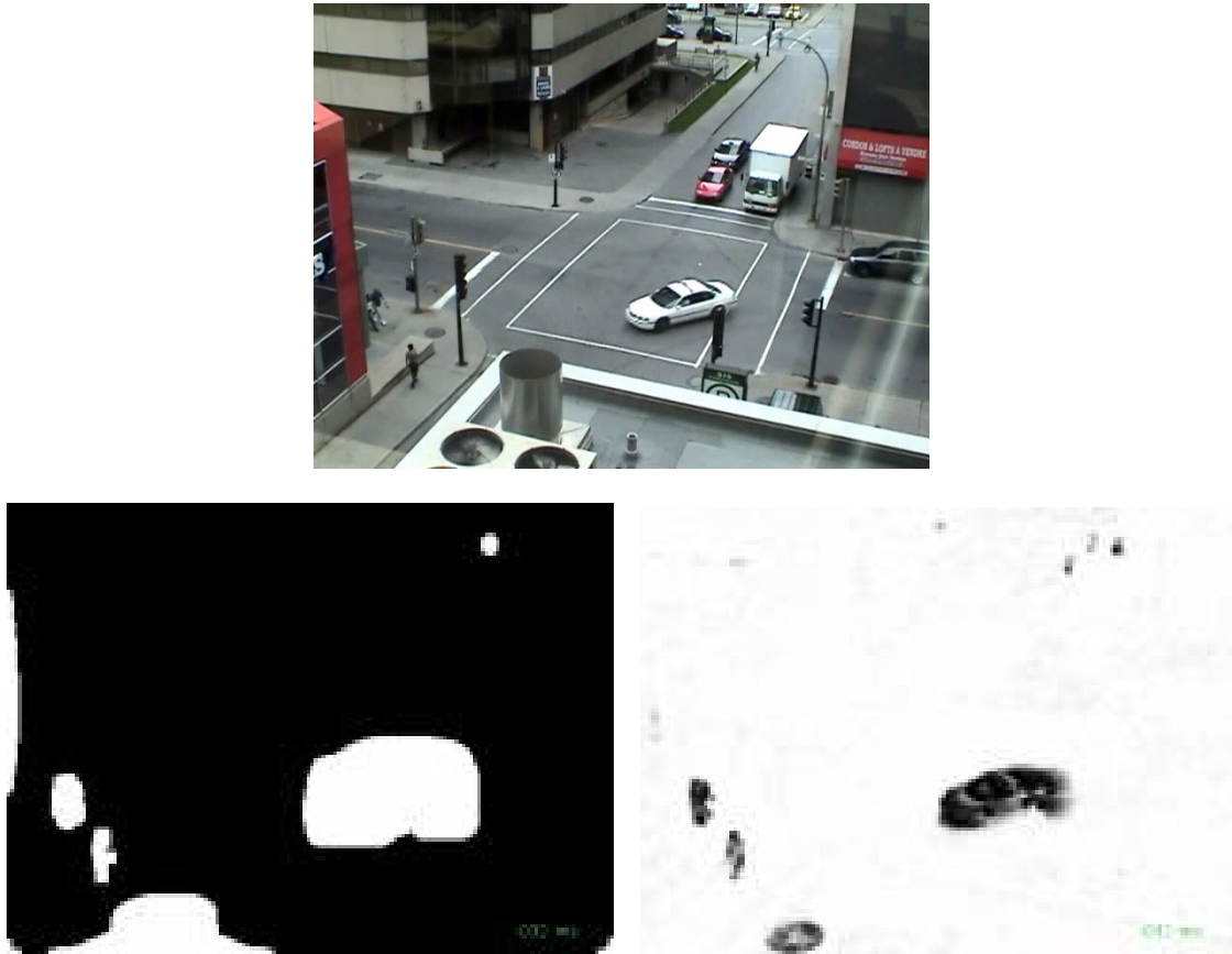
Figure 1: Input frame (top), its motion map (bottom-left) and the background probability map (bottom-right).
