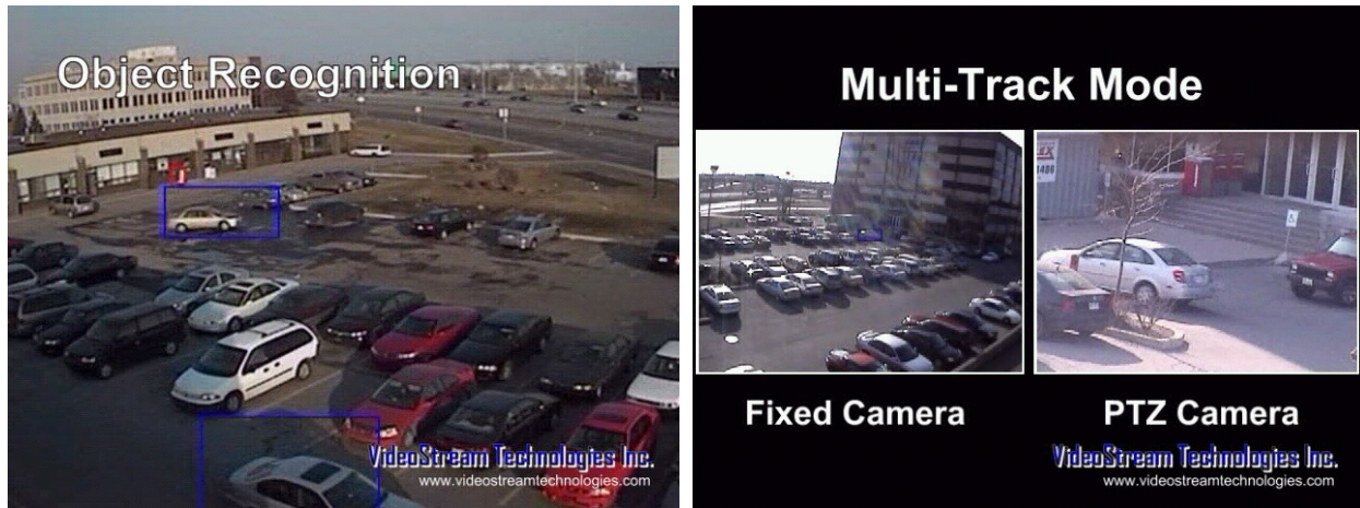
Figure 6: Two examples of fully operational uses after system integration. On the left-hand side, three moving objects detected and tracked: 2 vehicles and 1 pedestrian in the far field by nearby the building. On the right-hand side, a far field moving car detected in the parking (even through glass reflection) and tracked in light mode.
