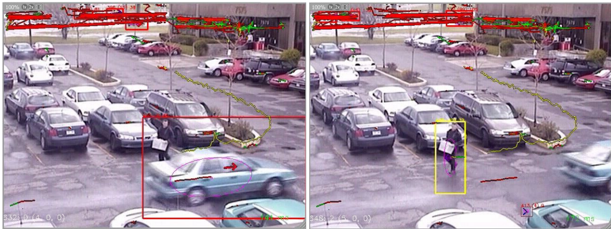
Figure 4: Two examples of detection, tracking and object recognition in the wide field mode on a parking lot. Human trajectories are in yellow, vehicles in red.
