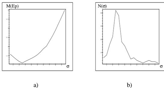
Figure 6: Results of the experiment for estimating the best value of the width  $\sigma$  to perform a smoothing. The experiment was performed for  $\sigma = 0.5$  to  $9.5$  with a step of  $0.5$  and  $\eta = 1$ . a) Mean error. b) Number of images that give rise to the minimum error.
