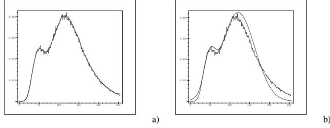
Figure 7: Radar image histogram estimation. a) Smoothing the histogram using the PNN approach with  $\sigma = 2.5$ ,  $MSE = 0.00026$ . b) Estimation of parameters by our model with  $K = 5$  and  $\beta = 0.97$ ,  $MSE = 0.0011$ .
