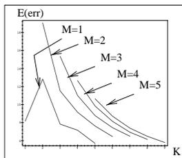
Figure 3: Average error  $E(err)$ , an indicator of the performance of the k-means algorithm, as a function of  $M$  and  $K$ .  $E(err)$  is calculated over 10000 histograms. A subset of 15000 points has been generated according to each histogram with different values of  $K$ , the number of clusters.
