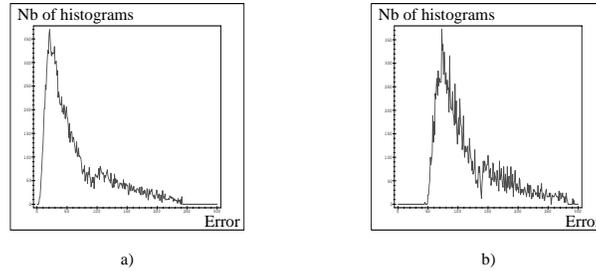
Figure 9: Frequencies of estimated histograms resulting with a given error  $\times 4.10^{-4}$ . a) Histograms estimated with our model (Average Mean Square Error:  $AMSE = 0.0132$ ), b) Histograms estimated with classical method (Average Mean Square Error:  $AMSE = 0.0308$ ).
